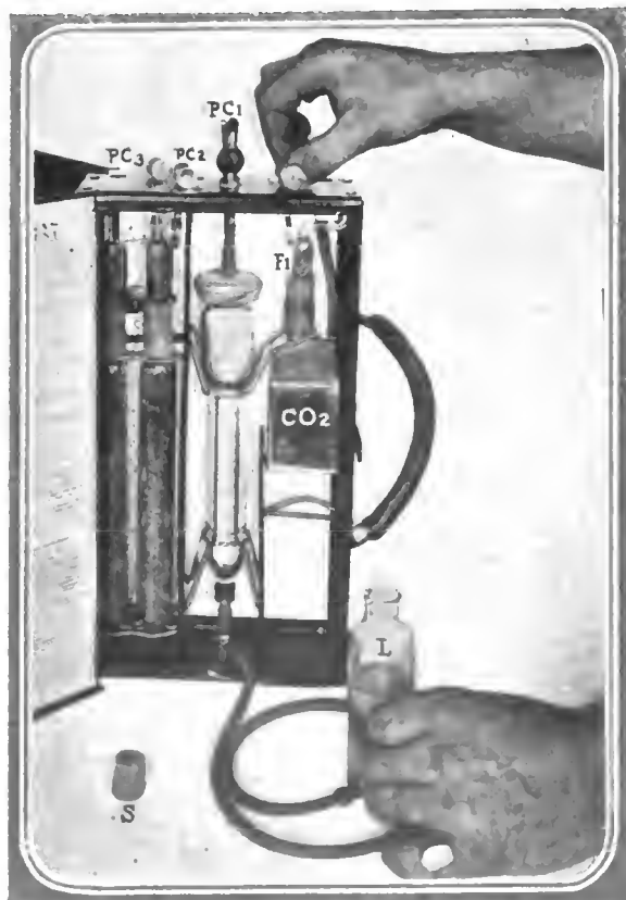
Fig. 2—Regulating the level of the caustic potash. With the cock closed tightly and pinch check held wide open, the leveling bottle is manipulated so as to raise the caustic to the top of the metal filling above the CO 2 chamber
